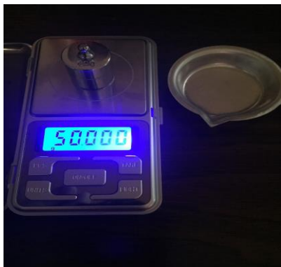
Figure 1. Frankford Arsenal Reloading Tools, DS-750 Digital Scale With 50.000g calibration weight. Powder cup right of scale.
