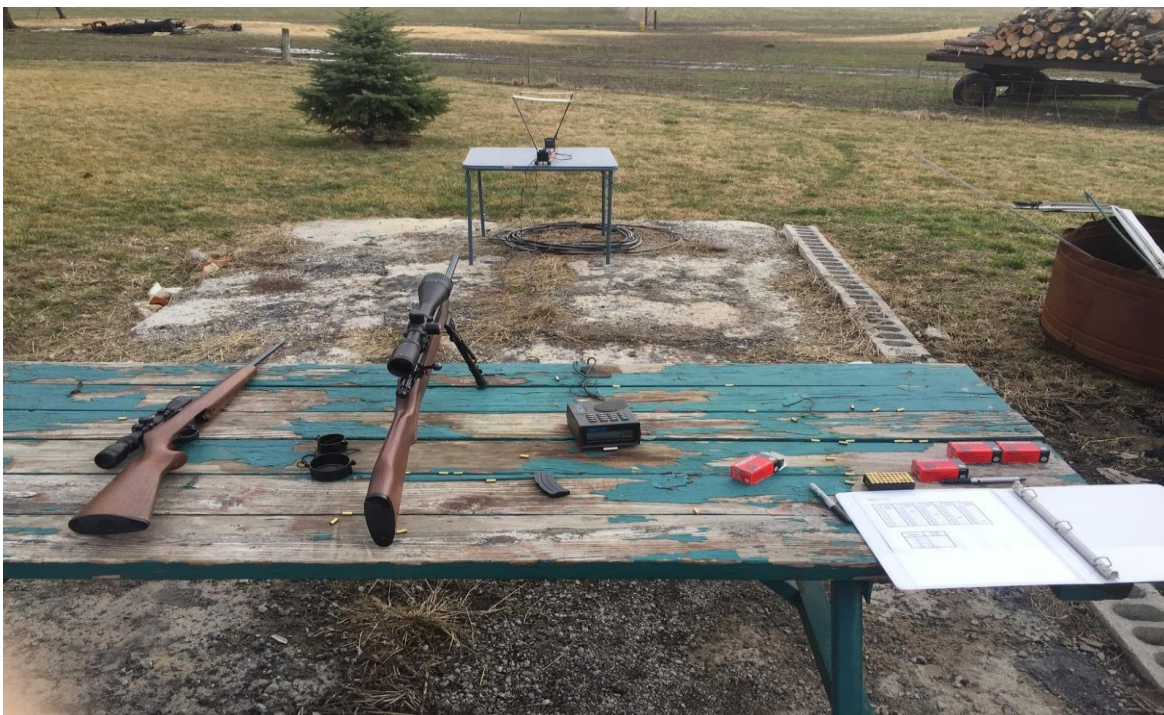
Figure 2, Testing Apparatus. The Firearm on the left is the Ruger 10/22, the firearm on the right is a Savage mkII with a Barska 8-32x50mm Rangefinding graph scope and bipod. The PACT chronograph is set up twelve feet from the muzzle of the barrel, and the chronograph display and timer is on the table communicating via a wired connection.
